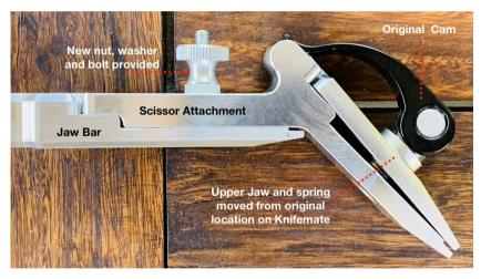
This attachment fits straight onto your Knifemate tool. Simply remove the top jaw and spring and install them onto the scissor attachment. A bolt nut and washer are provided to secure the attachment to your Knifemate tool. Remember do not over tighten the cam, you may damage the tool. Once the tool is assembled simply load your scissor blade into the tool, set the desired angle and commence sharpening.
