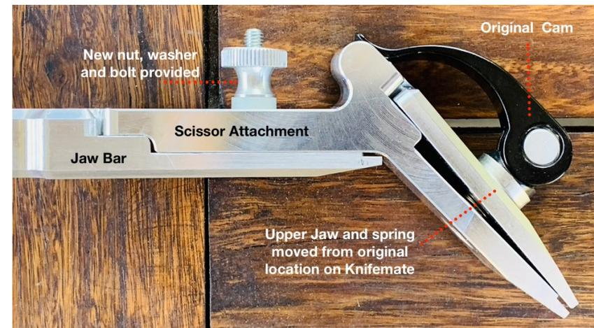
This attachment fits straight onto your Knifemate tool. Simply remove the top jaw and spring and install them onto the scissor attachment. A bolt nut and washer are provided to secure the attachment to your Knifemate tool. Remember do not over tighten the cam, you may damage the tool. Once the tool is assembled simply load your scissor blade into the tool, set the desired angle and commence sharpening.
